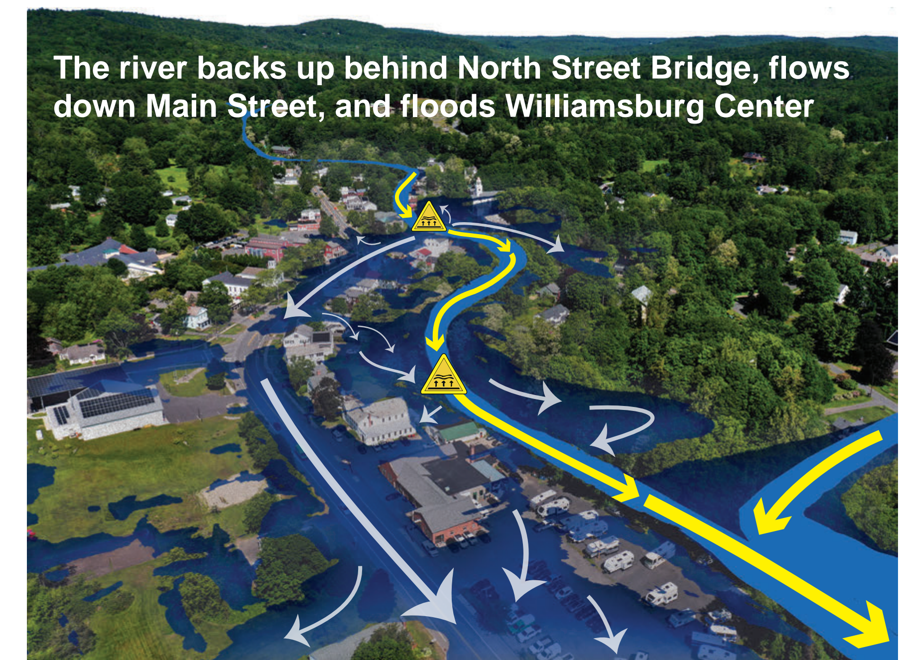
The river backs up behind the undersized North Street Bridge and overtops the channel
